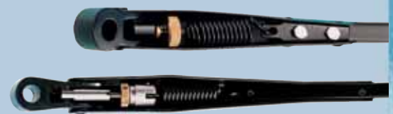
Gallery with adjustable spring pressure
